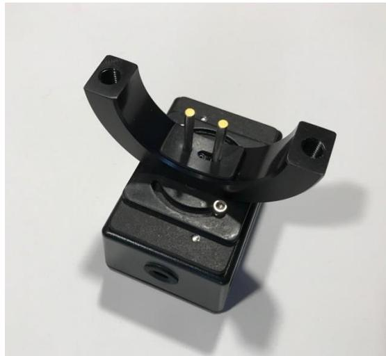
The pressure-sensing (PRS) option for the CDI 5400 flowmeters allows plant managers to monitor pressure throughout an air distribution system along with flow. A pressure sensor is mounted between the two flow-sensing probes. It accesses pipe pressure through a cutout in the gasket that seals the ring to the pipe.
