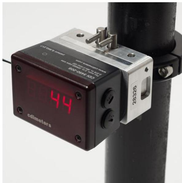
The CDI 5450 is a modified version of the 5400 model that allows installation under pressure. It incorporates two valves through which the probes pass and a muffler that collects chips from the drilling process. It takes an equal amount of installation time as our standard meters and requires no shutdown of the compressed-air system.
