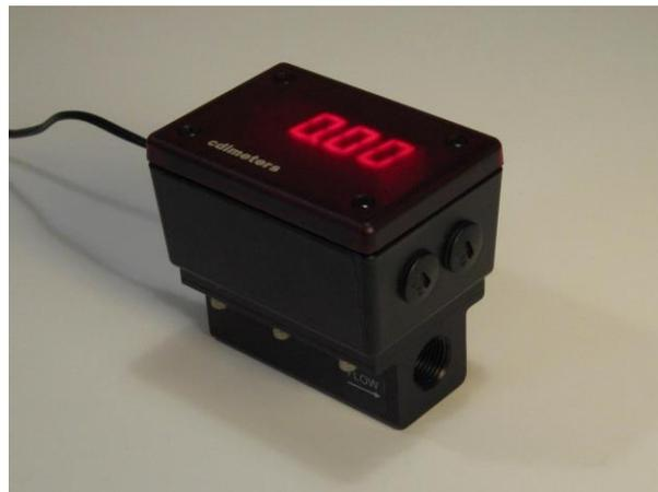
The CDI 5100 extends the capability of the CDI 5000 series to the low flow rates found in many point-of-use applications. It does this by concentrating the flow into a small area that is chosen to optimize the tradeoff between pressure drop and low-flow sensitivity. Used in its intended flow range and at a pressure of 100 psig, the 5100 will create a pressure drop no greater than one psi.
