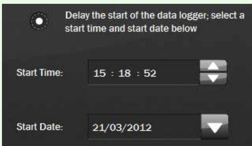
To start logging at a later time and date, select the Start Time (hh:mm:ss format) and Start Date (dd/mm/yyyy format) at which you want to start logging, then click finish.
