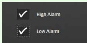
You have the option to set no, one or both alarms. The LEDs on the EL-USB-4 will flash in one of the ways listed below.
